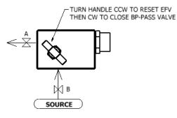
TO RESET CLOSE A OR B THE OPEN BY-PASS VALVE
